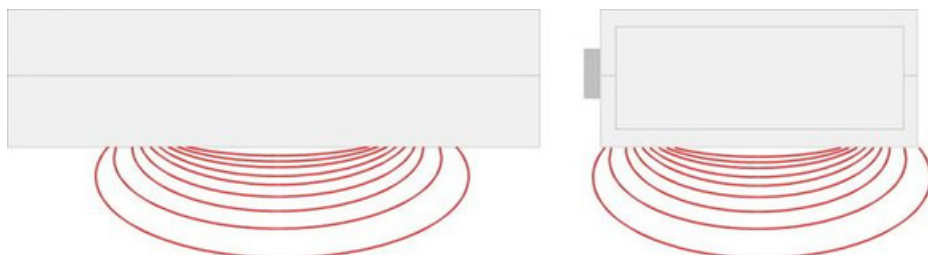
Side view: measuring field and penetration depth for "25 mm"
